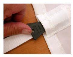
Insert the batten into the pocket.
