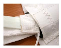
Use the batten tool to push the webbing-velcro tab into the batten pocket. The tool will prevent the velcro from sticking together.
