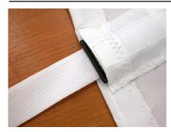
Be sure the batten is seated all the way into the pocket.
