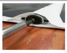
Use a screwdriver to tighten the adjuster. As you tighten the screw, the Rocket tensioner pushes the batten towards the luff and the 'ears' on the Rocket will be held by the small loop of line.
