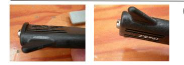
Rocket tensioners have a 'top' and a 'bottom.' The top side is the left photo with the lip that runs across the tensioner. The lip and 'fins' are used to hold the tensioner in place using a small small cord sewn into the sail. The top faces away from the sail.
