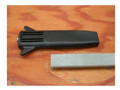
The RBS Rocket tensioner is a female fitting that holds onto the batten end. By turning the screw on the tensioner, the batten is pushed away from the tensioner, forcing the batten into the pocket.
