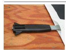
The batten fits into the pocket passing over the small cord loop on the sail side of the batten pocket.
